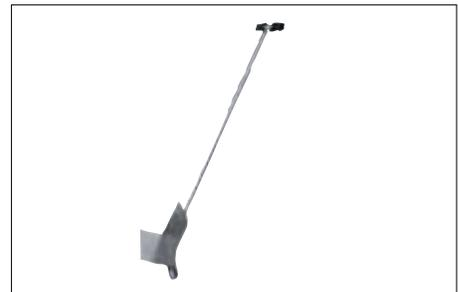
When using the DITRA-ROLLER, place a weight (e.g., bags of mortar/grout or box of tile) not to exceed 75 lbs on the DITRA-ROLLER shelf. Slowly move the roller from one end of the matting to the other, slightly overlapping successive passes.
